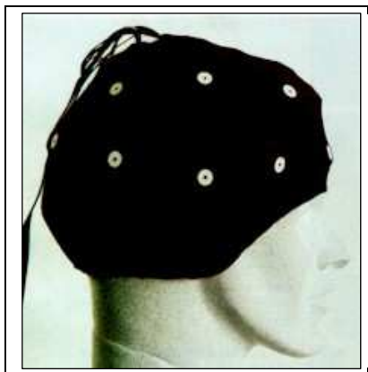
Fig. 2. Mindset MS-1000 EEG system Electro-Cap
