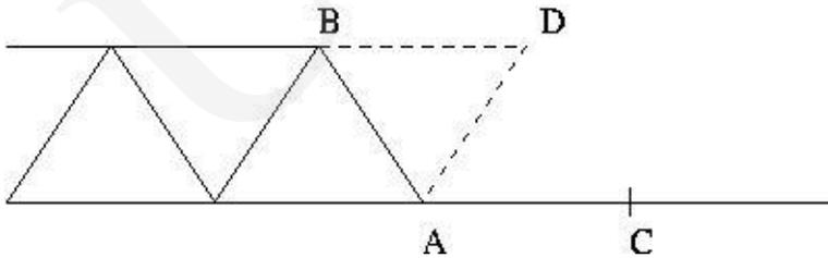
Fig. 2. New node construction when  $\alpha > 2\pi/3$
