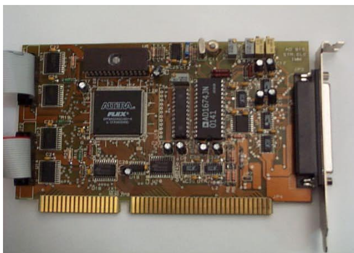
Fig. 3. The analog-digital card ADC615
