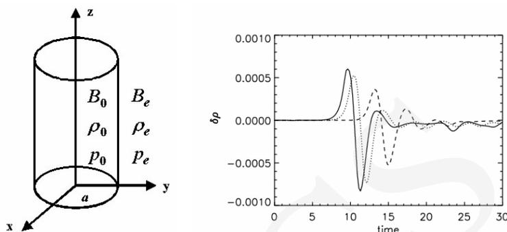
Fig. 7. A simple model of the geometry of a loop and time-signatures which are obtained by measuring the mass density at different detection points:  $x=0, y=0, z=0$  (solid line),  $x=0, y=0, z=4$  (dotted line),  $x=0, y=0, z=9$  (dashed line)
