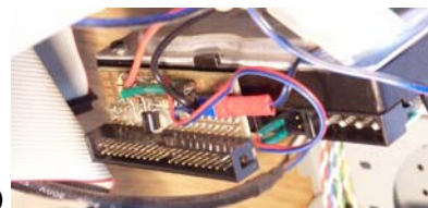
Fig. 4. Module of the HDD switch (a) and its placement in the computer (b)
