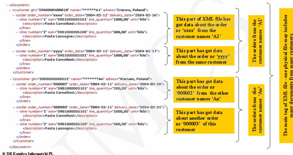
Fig. 2. The logical structure of the orders' XML file example - provided by firm A
