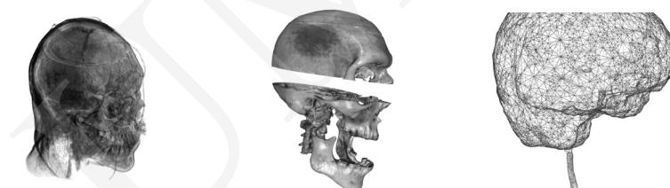
Fig. 6. Examples of three dimensional visualizations, from left: volumetric rendering, textured isosurface rendering, and isosurfaces rendered as triangle meshes
