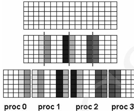
Fig. 1. Schematic view of 2D grid divided into 4 subdomains.
