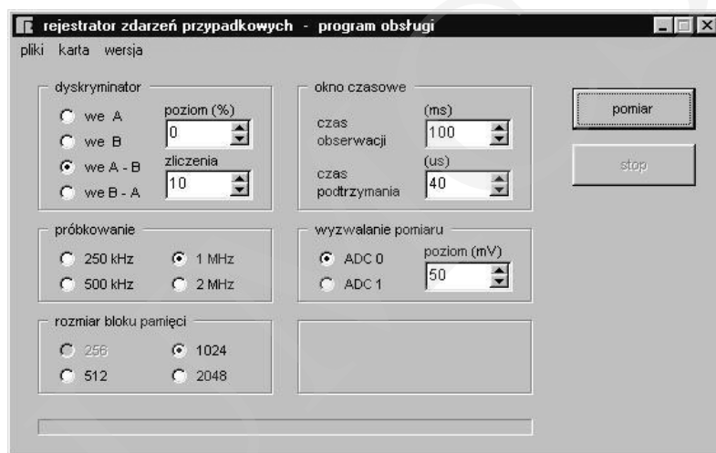
Fig. 6. Graphical interface for the recorder operation supervising program
