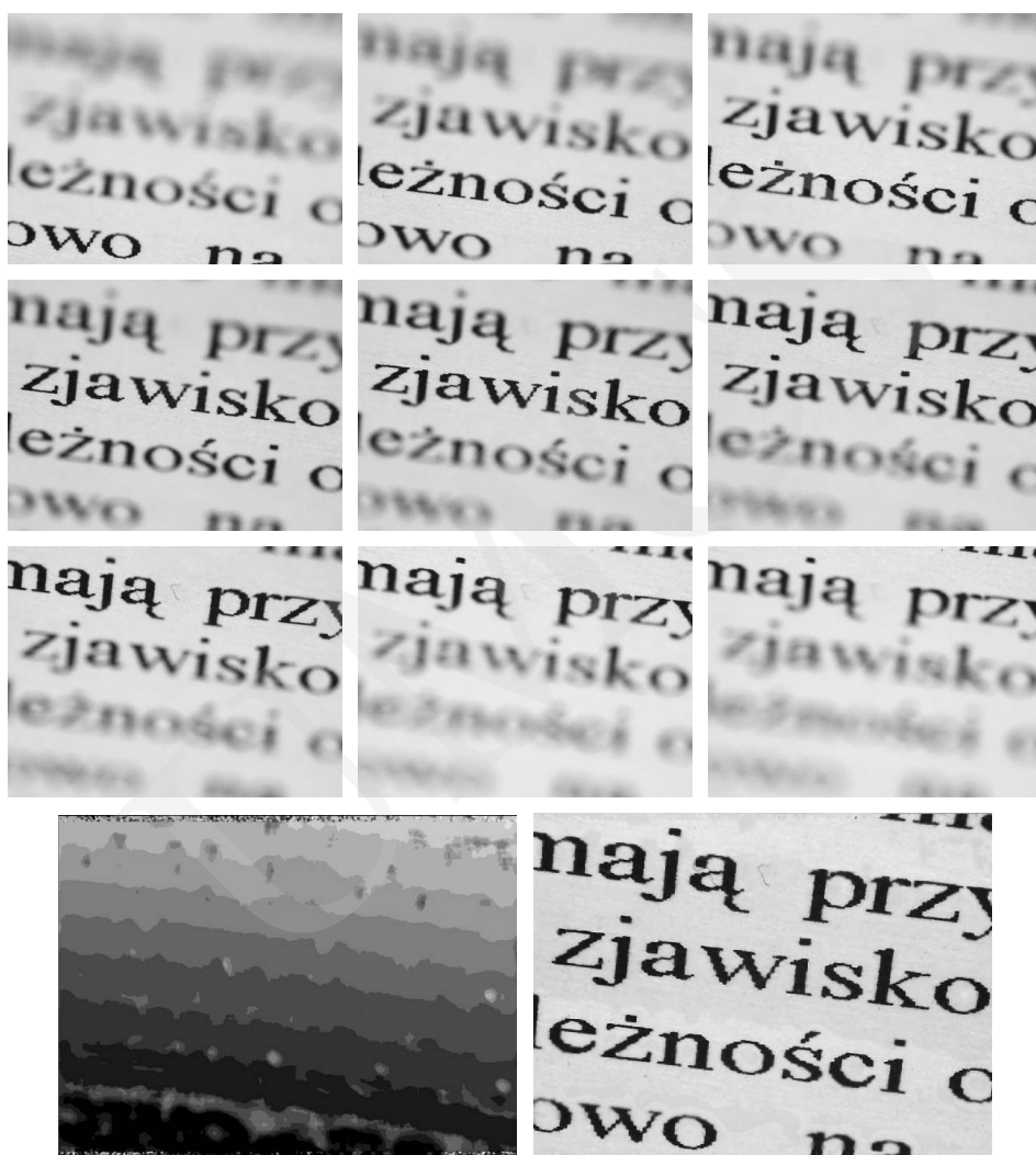
Fig. 7. An example of the whole series of images with the shallow depth-of-field problem with different focus length set (9 images at the top), depth map (bottom left) and reconstructed full focused image (bottom right)
