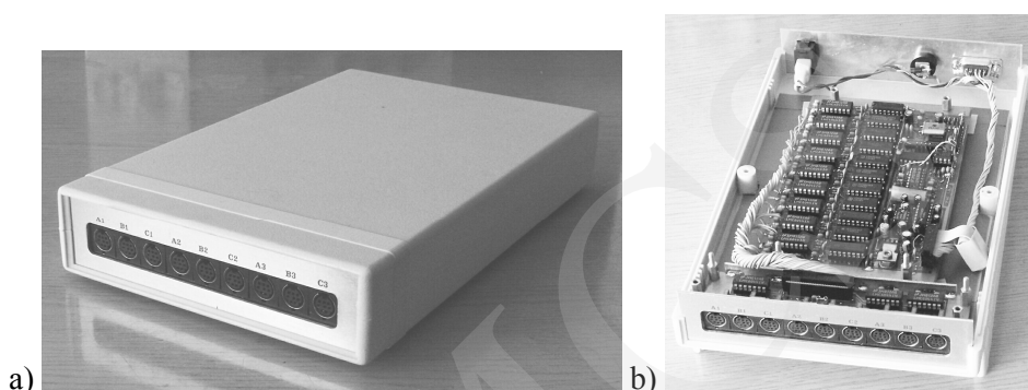
Photo 1. Recorder of curves I = f(U) : appearance of the recorder (a) and its interior (b)
