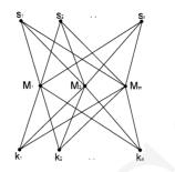
The degree of cohesion of the graph equals d = |E| - |V| + 1 = rm + nm - r - n - m + 1 = (r + n - 1)(m - 1). If we compare this topology with the previous one (in the previous topology m = 1 and d = 0), the degree of reliability increases *m*-1 times for this SK. The algebraical notation for this topology:
