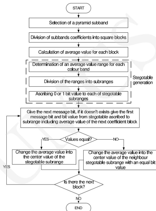
Fig. 2. Steganographic algorithm
