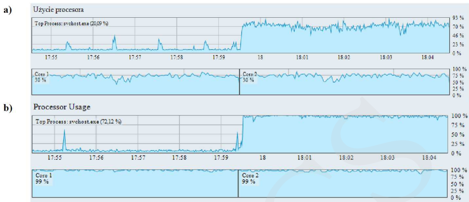
Fig. 11. The CPU usage for the VPN tunnel with SSTP/IPsec in FastEthernet: a) server; b) client.
