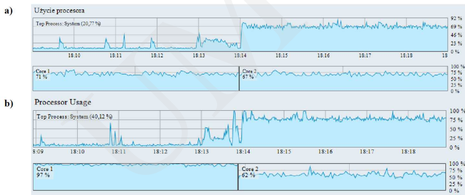
Fig. 12. The CPU usage for the VPN tunnel with IKEv2 in FastEthernet: a) server; b) client.
