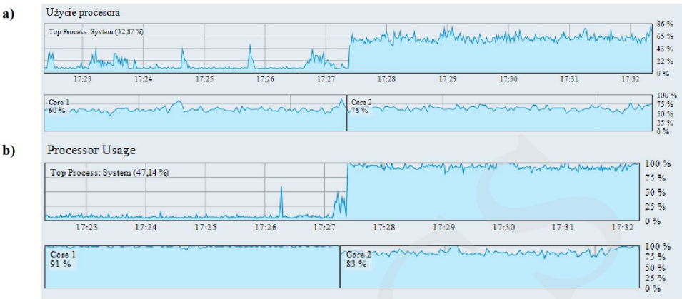
Fig. 9. The CPU usage for the VPN tunnel with PPTP/IPsec in FastEthernet: a) server; b) client.
