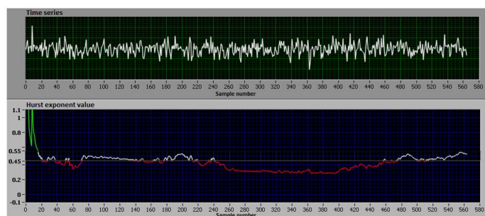
Fig. 4. The charts of the network delays for the VoIP traffic with a heavy load and the Hurst exponent value obtained using the absolute value method.
